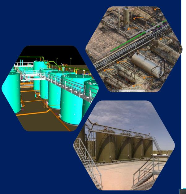
SCANNED SICK METER SPOOL PIECE AND MODELED WITH EXISTING PIPING
